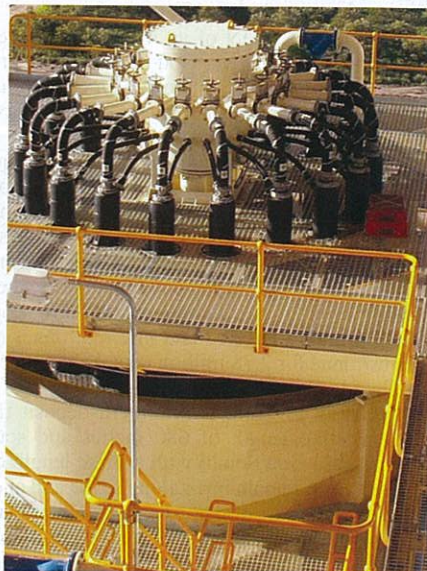
Two B6000/20 Jameson Cells will be used at the Ukhaa Khudag coal project.
