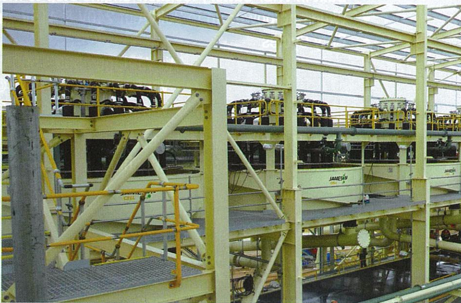
The Xstrata Technology Jameson Cells commissioned at Yancoal Australia's Moolarben Coal Operations.
