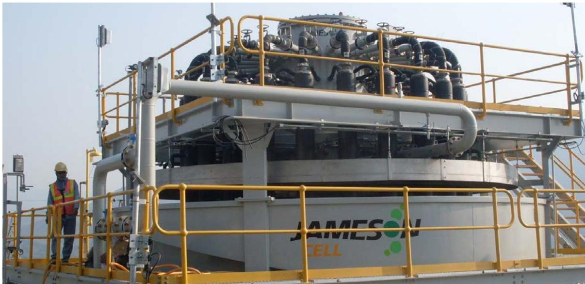
*Jameson Cells can perform all duties in a flotation circuit and will now comprise the entirety of a new circuit at Hudbay's New Britannia.*
